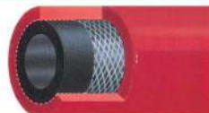
WELDING HOSE (OXYGEN OR ACETYLENE) – SINGLE HIGH TENSILE SYNTHETIC TEXTILE BRAIDED SYNTHETIC RUBBER HOSE FOR INDUSTRIAL WELDING WITH OXYGEN OR ACETYLENE – WP 20 BAR
