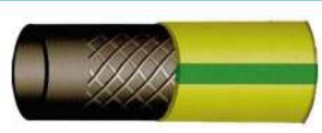
PVC GARDEN HOSE PVC COMPOUND SYNTHETIC TEXTILE REINFORCED HOSE FOR GARDENING AND GENERAL WATER DISCHARGE SERVICES – WP 3 TO 6 BAR
