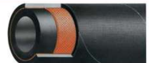
SAE 100 R6/ EN 854 R6 FOR HYDRAULIC CONTROL LINES, DISCHARGE UNDER LOW PRESSURE OF HYDRAULIC FLUIDS, FUEL OIL, GREASE, AIR AND WATER (20 to 34 BAR)
