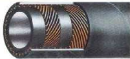
RADIATOR HOSE – WP 4 BAR HEAT AND ANTI-FREEZE LIQUID RESISTANT EPDM RUBBER HOSE FOR CONVEYING HOT WATER IN COOLING SYSTEMS, AUTOMOTIVE AND STATIONARY ENGINES
