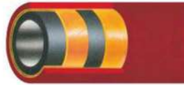
STEAM HOSE – WP 17 BAR, 2000 C STEEL WIRE REINFORCED SATURATED STEAM EPDM RUBBER HOSE FOR SERVICES IN CHEMICAL PLANTS, STEEL MILLS, REFINERIES, SHIPYARDS AND ALL INDUSTRIES
